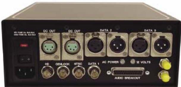
Ruggedized CA5442X custom package, designed for Fletcher Chicago, brings AC power input, DC output and a connector set specially adapted for HD sports production
